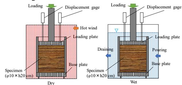
Fig. 1. Schematic diagram of drying-immersion compression apparatus.
