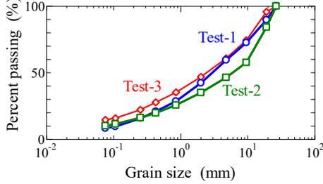
Fig. 4. Grain size distribution of specimens after shearing.
