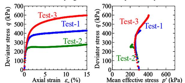
Fig. 3. Results of undrained triaxial compression test.
