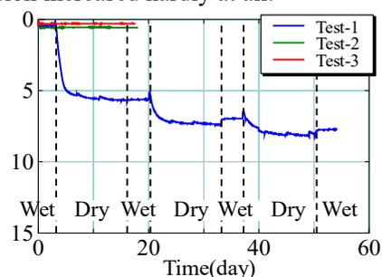
Fig. 2. Relationship between compression strain and time for Tests 1–3 across the drying-immersion compression cycles.
