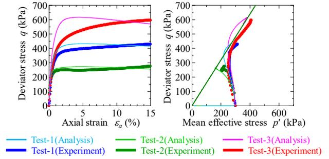
Fig. 5. Simulation of undrained shear tests.
