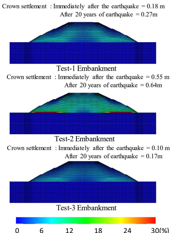
Fig. 8. Shear strain distribution 20 years after the earthquake.
