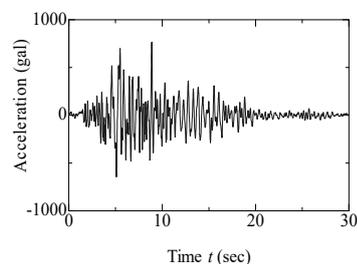
Fig. 7. Input seismic motion.
