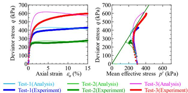
Fig. 5. Simulation of undrained shear tests.
